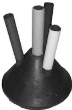
Each tube is between 20cm and 30cm long, made of plastic with an internal diameter of 2.3cm and an external diameter of 3cm.
