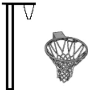
A 30cm deep net attached to a 20cm diameter hoop and closed at the bottom, fixed at the top of a vertical stand so that the top of the net is 2m13 above the ground. The stand may be fitted with either a metal spike or some other form of stabiliser to hold it securely upright and to maintain the net in position facing the riders.
