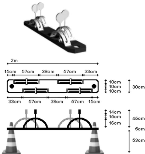
The point at which the target disc is attached to the pivot arm and the pivot mechanism at the bottom of the arm are subject to very high impact forces and must be strong and well constructed.
